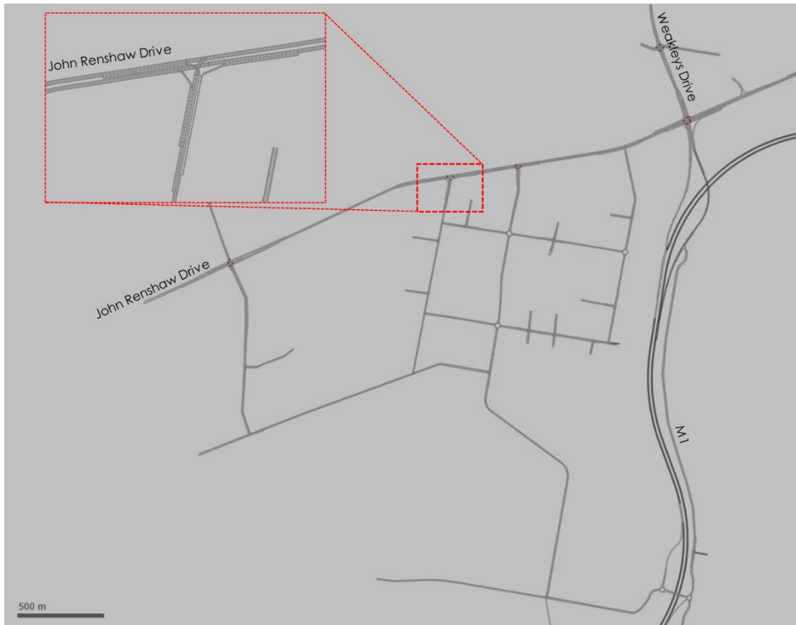
Figure 6.10: John Renshaw Drive with three new signalised intersections
